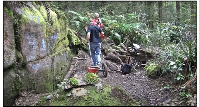
Fig. 1. People undertaking ground penetrator radar investigations in front of the original Kaimanawa Wall (producing the reflection profile in Fig. 6). Note the unnatural flat-floored depression in front of the wall and the lack of scree along its base.
