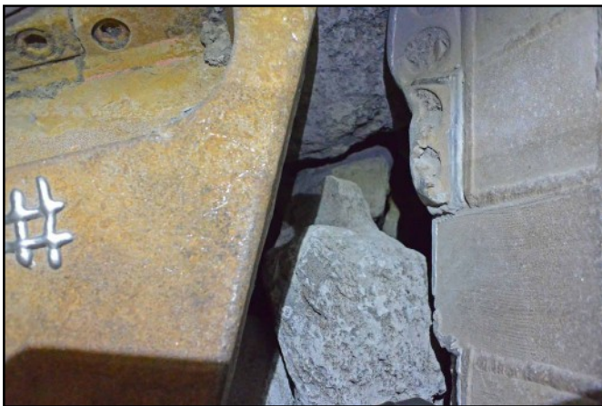
Fig. 5. Void 2 - solid basalt boulder in grinder.
