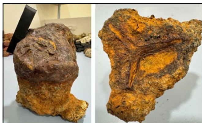
Fig. 9. Highly magnetic triangular iron rebar farm fencepost ... not a meteorite (pers. obs.).
