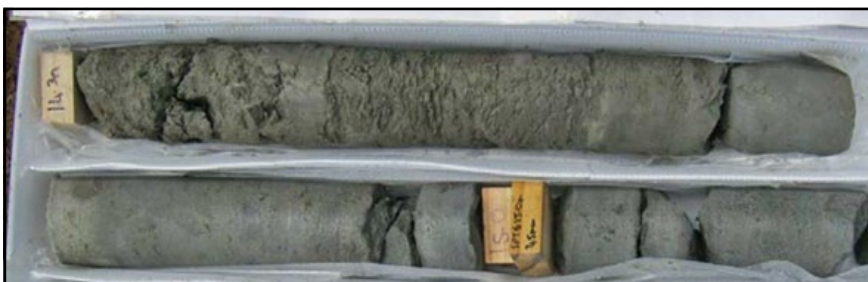
Fig. 2: Excerpt from photo accompanying log (from NZGD 64633), showing the transition from sheared Allochthon to competent Pakiri at 14.5m.
