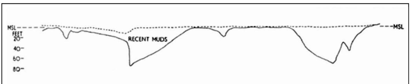
Fig. 6. East (left) to West (right) cross-section across Hobson Bay along the route of the former sewerage line. The solid line is the top of the Waitemata Sandstone and the pre-12000 years ago topography, whereas the dotted line is the present day surface of Holocene mud that now fills Hobson Bay. From Auckland Drainage Board in Searle (1959).
