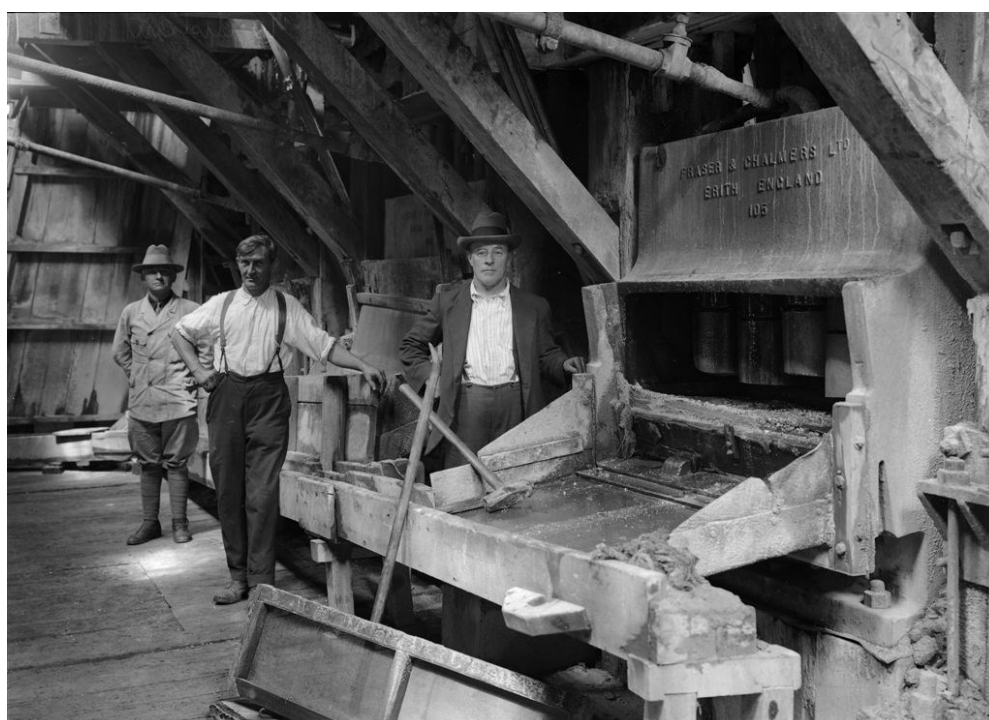
Figure 7. Mortar box with the front removed, showing five stamper shoes. The quartz ore mixed with water was pounded by the stampers to produce a slurry. Alexander Turnbull Library, ½-233105-G
