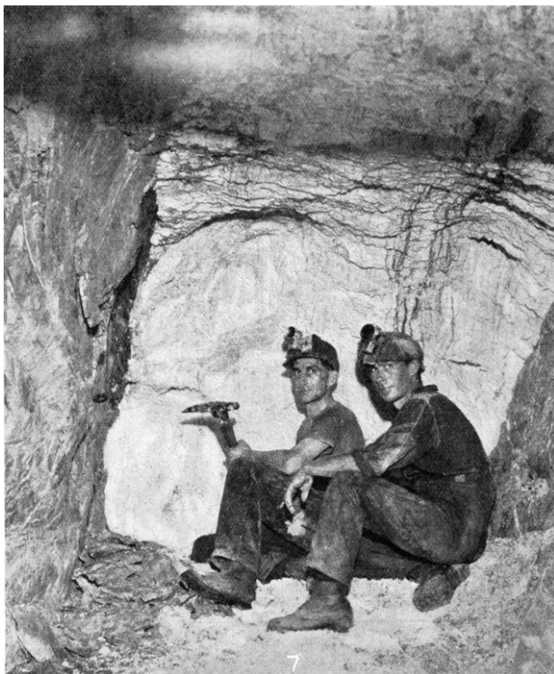
Figure 3. Quartz reef (white), locally up to 1.7 metres wide, at no 14 level in the Blackwater mine, with darker greywacke country rock on both sides.
