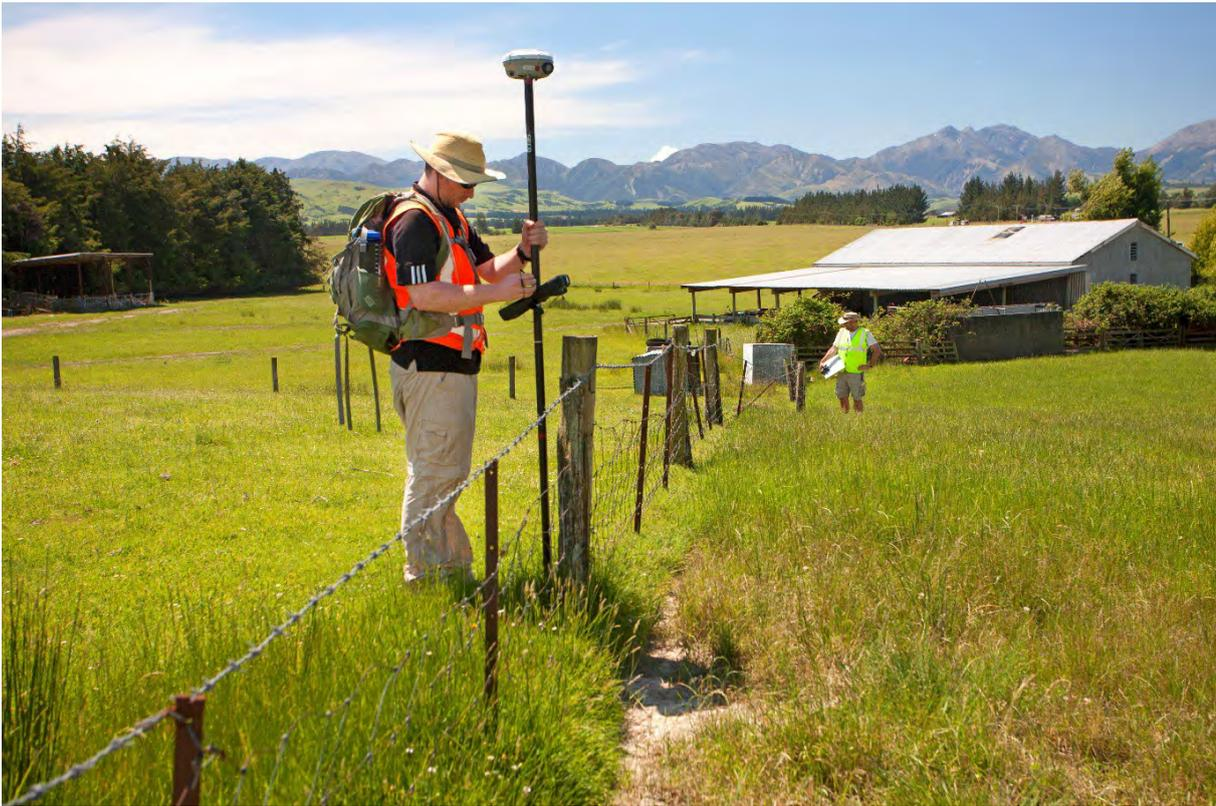
Figure 6. Photograph (looking north) of displaced fence on The Humps Fault, Dalmer Property, near Waiiau (Photograph Kate Pedley).
