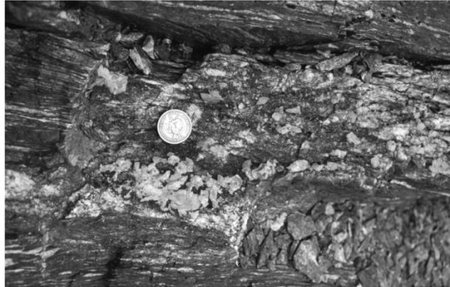
**A:** Euhedral quartz and calcite crystals on surface of sub-horizontal fracture
