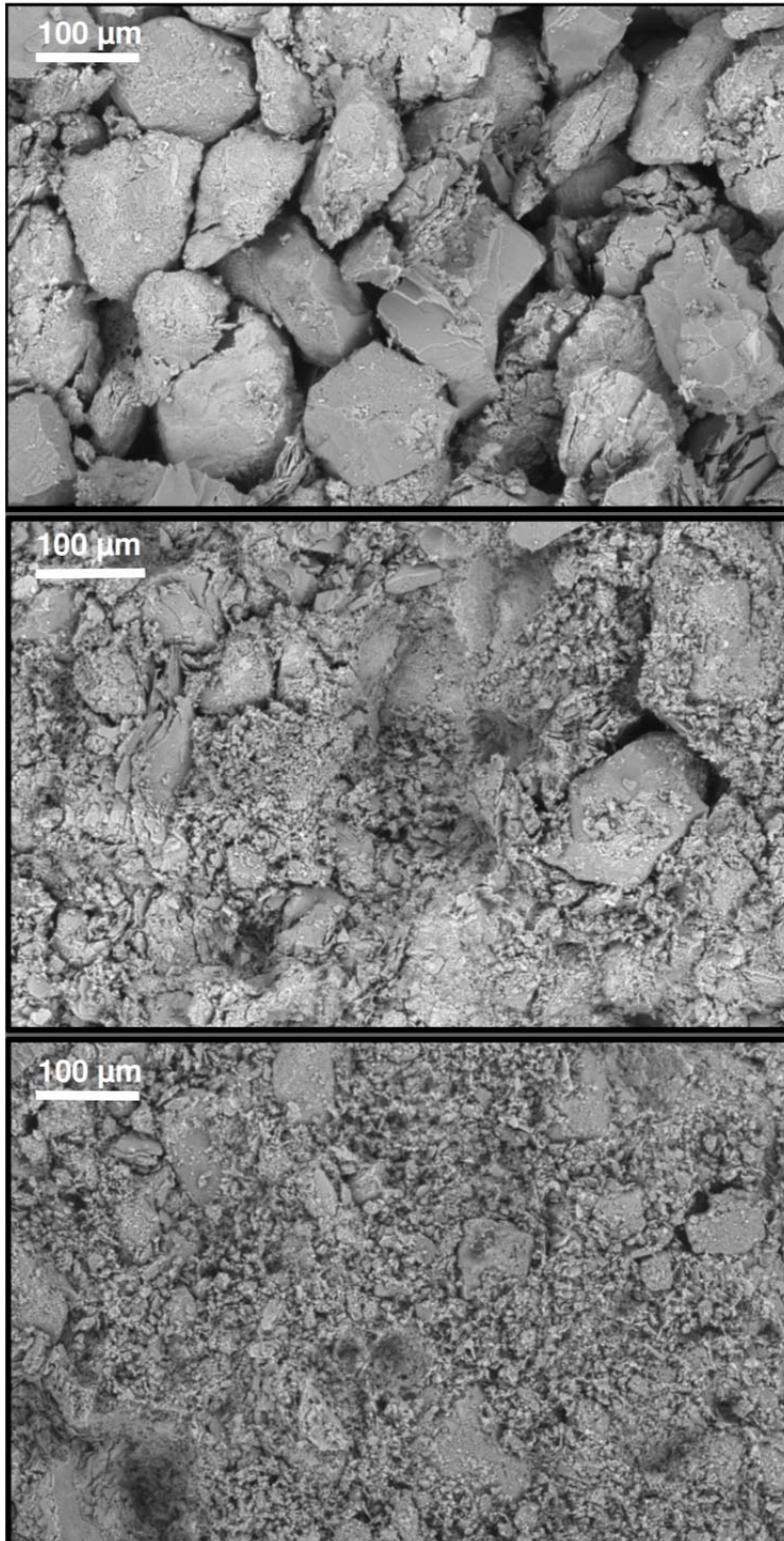
Figure 10. SEM images of unfaulted (top image) and faulted (middle and lower images) sandstone from the Mount Messenger Formation in the Tongaporutu River coastal section. The middle image is from a faulted sandstone with 1 mm of displacement and the bottom image a fault zone in a sandstone after 65 mm of fault displacement. Note the rapid initial destruction of the sandstone grains after  $\sim 1$  mm of displacement.
