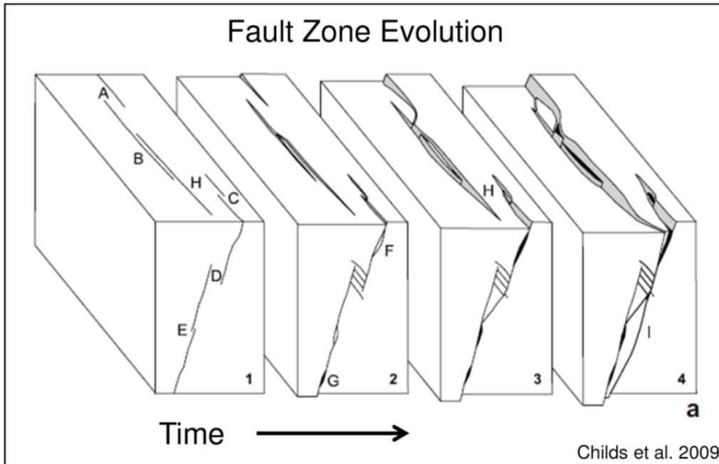
Figure 7. Block diagram illustrating the evolution of a fault array with increasing displacement at times 1 to 4. Individual fault irregularities, either asperities or segment boundaries are labelled A to I. Figure modified from Childs et al. (2009).
