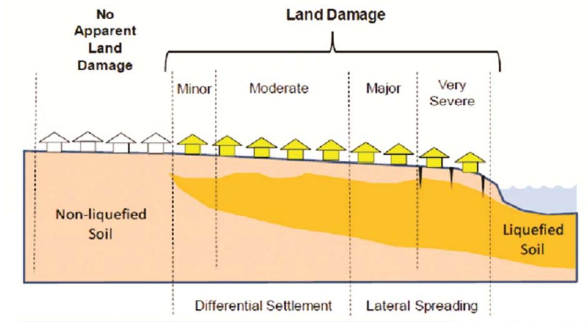
**Figure 3:** Schematic cross section of the spatial distribution of liquefaction induced land damage zones as observed following the September and February events (Jacka & Murahidy, 2011).
