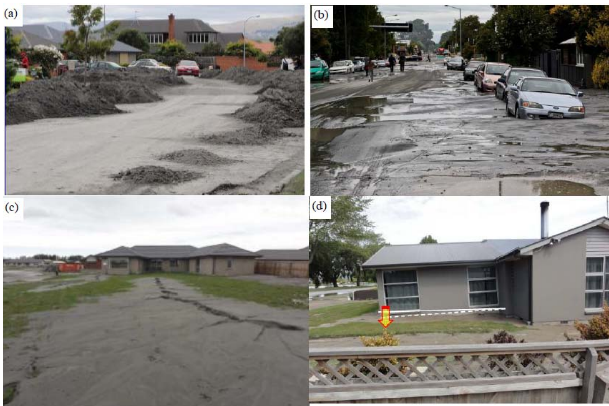
Figure 17 Typical manifestation of liquefaction in residential areas (Fig. 19 from Cubrinovski et al. 2011)
