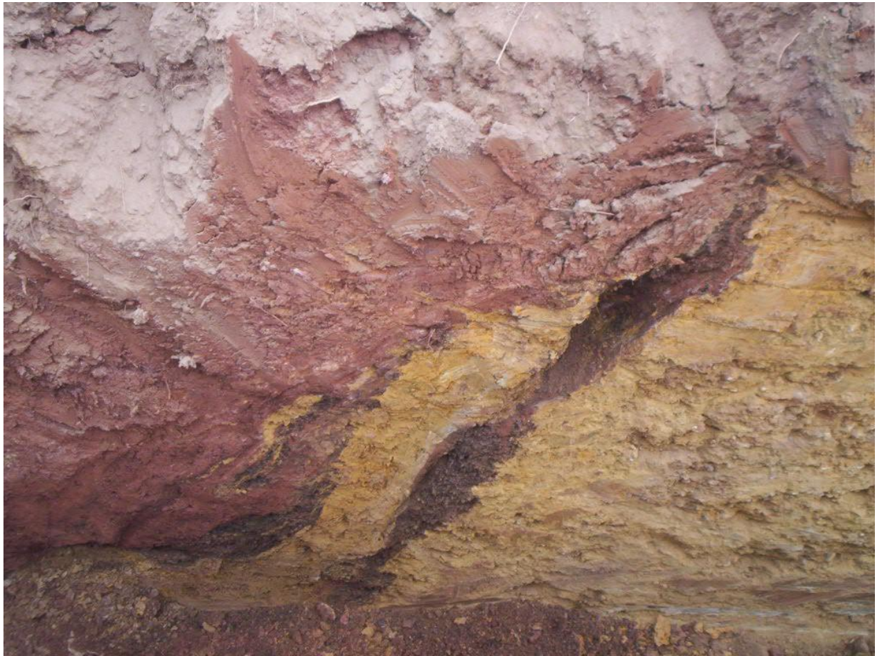
Figure 8.1 Eastern strand of Flaxmore Fault in trench at Bishopdale Subdivision, Nelson. Red clay is sheared Bishopdale Formation and yellow material is Port Hills Gravel. Black material is manganese oxide on fault shears.
