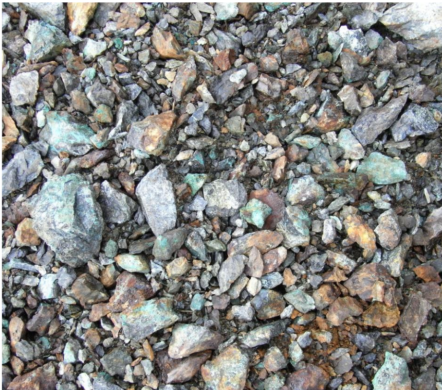
Figure 4.15 Champion Mine ore consisting of malachite coating serpentinite, weakly cupriferous pyrrhotite and sparse small fragments of native copper.
