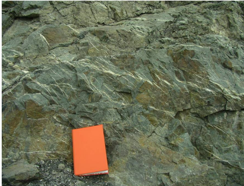
Figure 8: En echelon array of extensional veins in sandstone. SE abutment of Benmore Dam. Field book is 20cm long. Viewed towards the SE.
