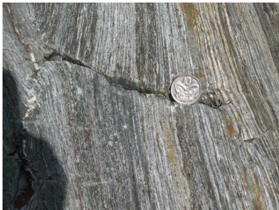
(e) late-stage subhorizontal open fracture
