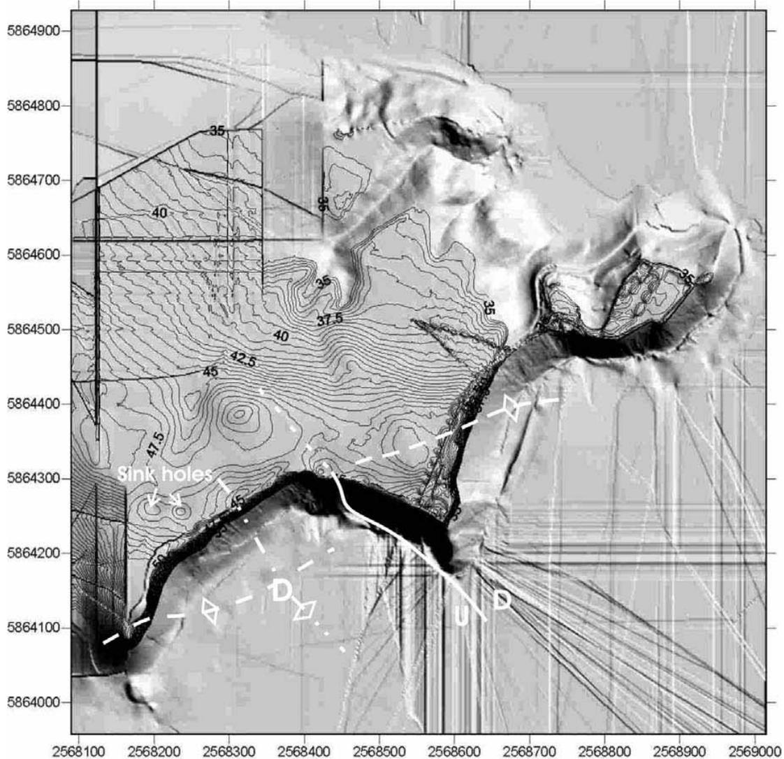
**Figure 9:** DEM of uplifted marine terraces showing contouring the terrace surface at 0.5m intervals. elevated areas on the T4 surface coincide with the crest of the Atia Anticline the northwest side of the Spaniards Bay Dome truncated by the cliff and along strike on the upthrown side of the fault on the north side of the bay separating the two domains.
