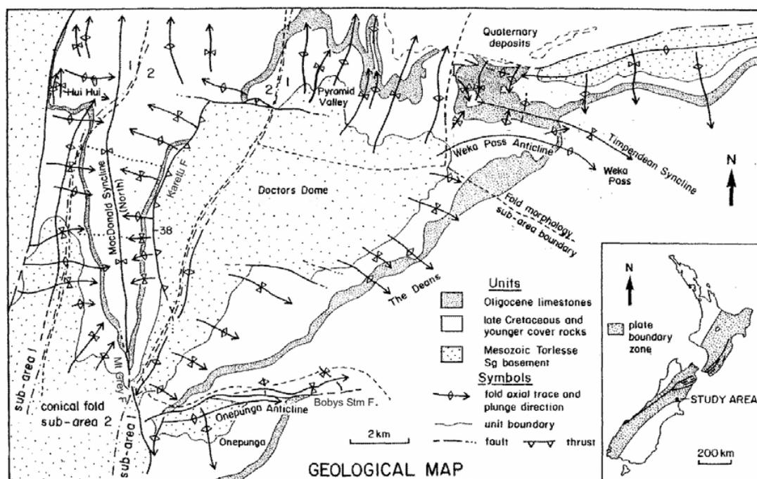
**Figure 2:** Structure of the Doctors Dome area. Fold details were derived by structure contouring the unconformity at the interface between Torlesse basement rocks and the cover sequence and the top of the Oligocene limestones. (map from Nicol, 1991)
