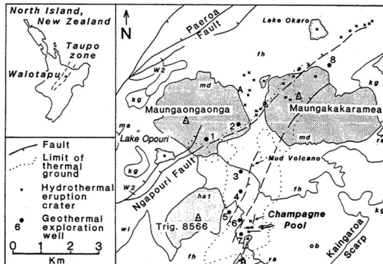
**Figure 10.** Simplified geologic map of the Waiotapu area; the unit abbreviations are keyed to Table 2. Also shown are the locations of drillholes (numbered) and hydrothermal eruption vents. From Hedenquist and Henley (1985).
