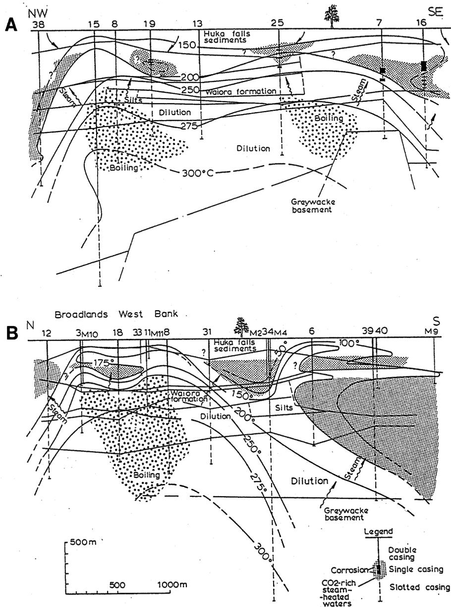
**Figure 8.** Northwest-southeast (a) and north-south cross-sections (b) through the Broadlands-Ohaaki system. Stipple pattern shows the distribution of CO<sub>2</sub> rich steam-heated waters; isotherms are also shown. From Hedenquist (1990).
