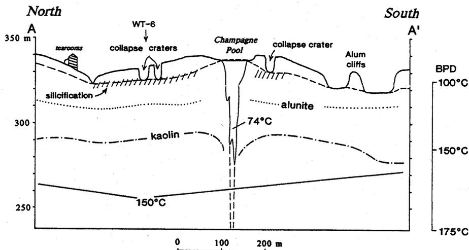
Figure 15. North-south cross section through the collapse crater-Champagne Pool vicinity, showing the water table and subsurface distribution of alunitite and kaolinite. BPD is boiling temperature at depth indicated.
