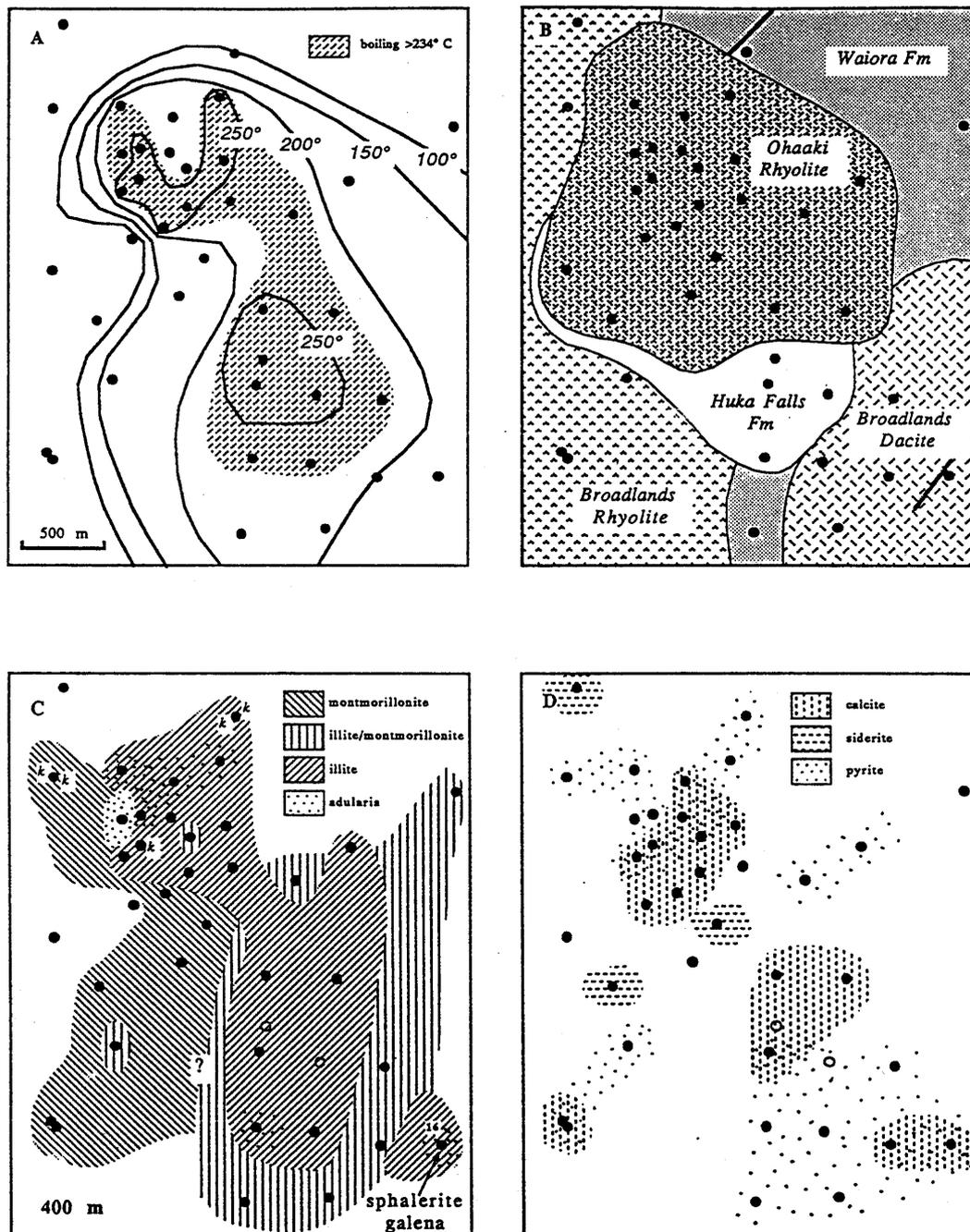
**Figure 9.** Plan views depicting, at approximately 400 m below the surface: A) temperature distribution and boiling zones, B) geology, C) clay and adularia distribution [k denotes occurrence of kaolinite], and D) carbonate and pyrite distribution.
