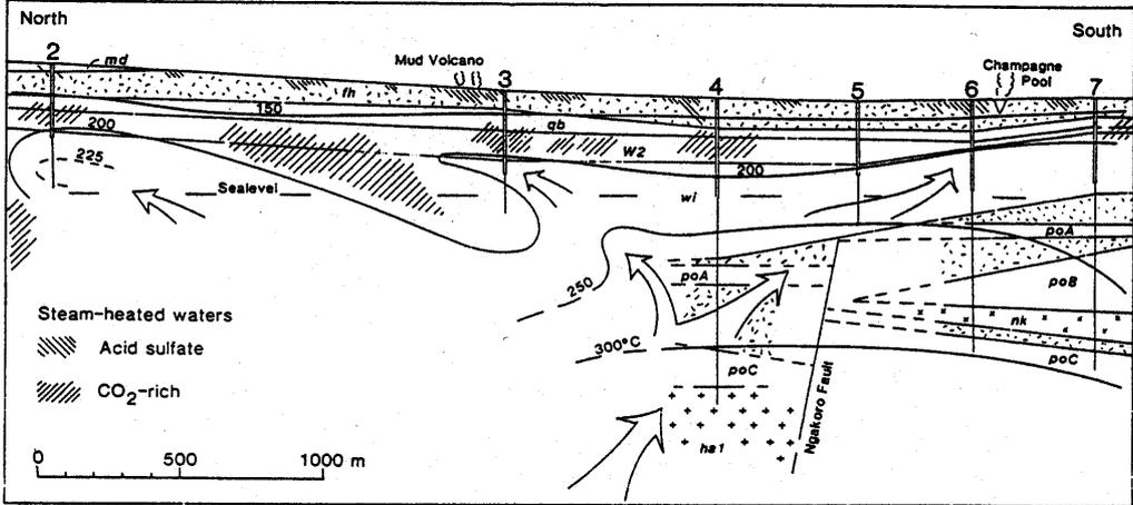
Figure 12. North-south section through the Waioatapu system, showing the geology, distribution of steam-heated waters, isotherms and flow paths of thermal fluids. (Hedenquist and Browne, 1989). Stratigraphic symbols keyed to Table 2.
