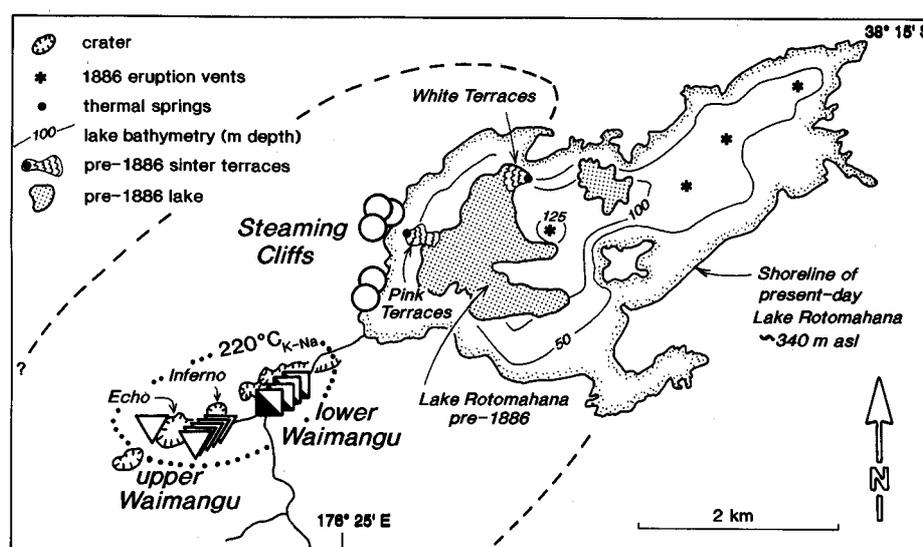
**Figure 17.** Location of present day thermal features and their relationship to the Pink and White Terraces and the pre-1886 Lake Rotomahana. The dashed line represents the 10 Ωm resistivity boundary (current electrode spacing 1100 m) delimiting the subsurface region occupied by chloride waters (Bennie et al., 1985). Dotted line represents 220°C isotherm based on K-Na geothermometer.
