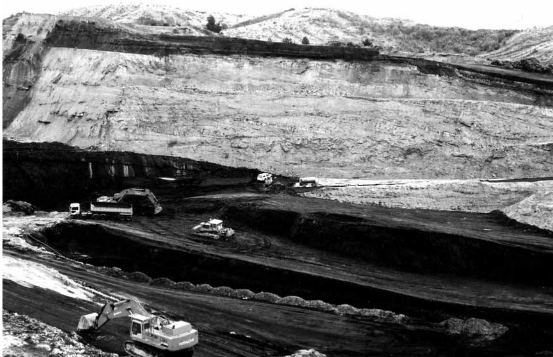
Figure 1.4 Kai Pont opencut mine, 1994. Highstand systems tract, incorporating Kaituna Seam (lowermost); 20m thick (highwall) interval of fine grained (sandy and muddy) sediments with high sinuosity channel forms (ECS sets) crevasse splay and flood-basin features; and the overlying Barclay Seam.
