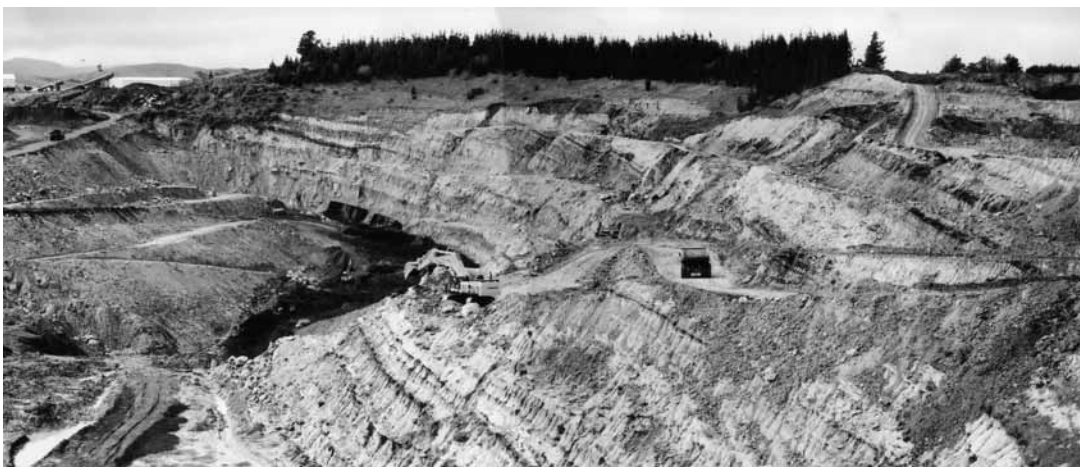
Figure 5.1 Ohai No. 16 opencast extension, October 2003. Production is from the Morley No. 2 seam on the pit floor. Morley No. 1 and Star Seams outcrop higher in the highwall (far right), and are overlain by Beaumont Formation.
