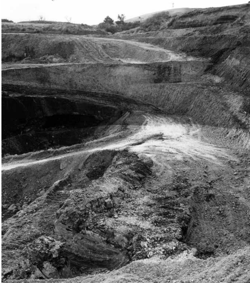
Figure 6.1 Nightcaps mine, May 1997. View north, showing exhumed roof of UM1 Seam (Morley Formation) adjacent to the eastern highwall (right of photo). The regional unconformity is defined on the surface between the coal roof and the overlying greenish conglomerate bed. Beaumont Formation sediments overlie the Morley Formation and are represented uppermost in the section by a coal seam (upper right).
