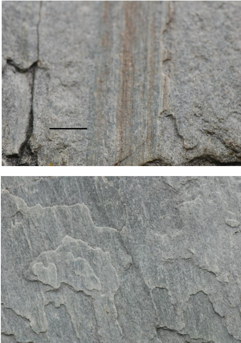
Fig. 7.2. Greenschist, two of many blocks used to make up the stone walls around the petrol pump near The Hermitage, showing the rock in cross-section (above) and in surface view (below). Scale bar 10cm approx. The rocks were brought in from the Wanaka area and are judged to be sedimentary in origin.
