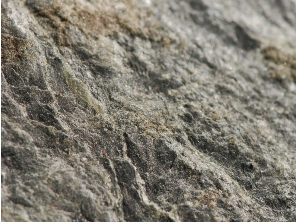
Fig. 1.10. Surface view of schist (the same sample as in Fig.1.9). Note the silky or lustrous appearance.
