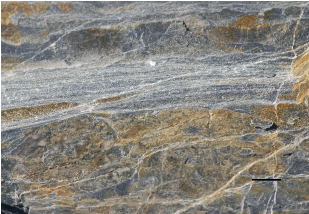
Fig. 1.9. Detail of schist rock, showing the fine layers due to reoriented and newly grown minerals under shear strain or directed pressure. This sample is from the Walpole Formation in the Mueller valley. Scale bar 1cm long.
